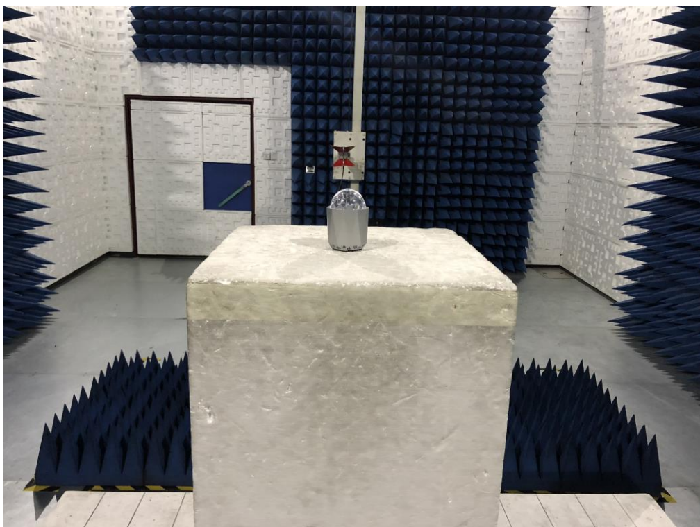
RADIATED EMISSION TEST SETUP ABOVE 1GHZ
