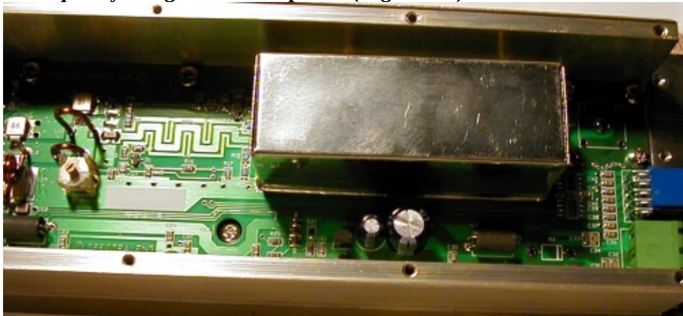
F Frequency Range Power Amplifier (Right Side) with Low Pass Filter Shelding
