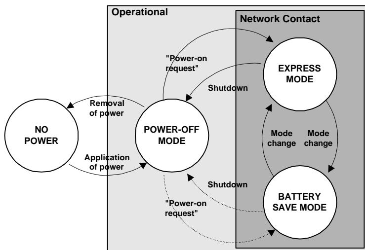
The NMX920 operates in one of three distinct power modes while power is applied to the **External Interface**; **POWER-OFF MODE**, **BATTERY SAVE MODE** and **EXPRESS MODE**. To provide control over the operational state, and power consumption of the NMX920, the OEM can change between these modes by issuing certain MASC commands and/or electrically activating the **DTR** line on the **External Interface**.
