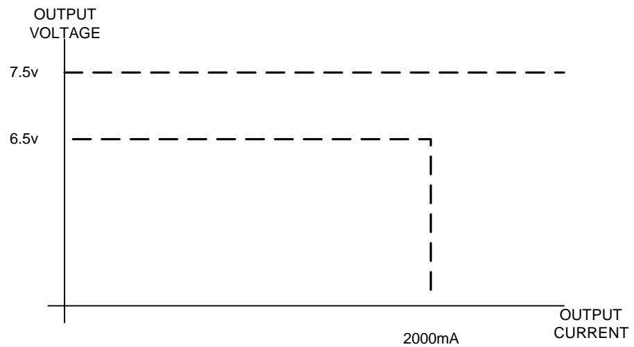
The output voltage must stay within these limits for any transient load change greater than 10uS.
