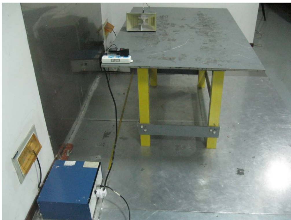
Conducted Emissions Test Setup - Side View
