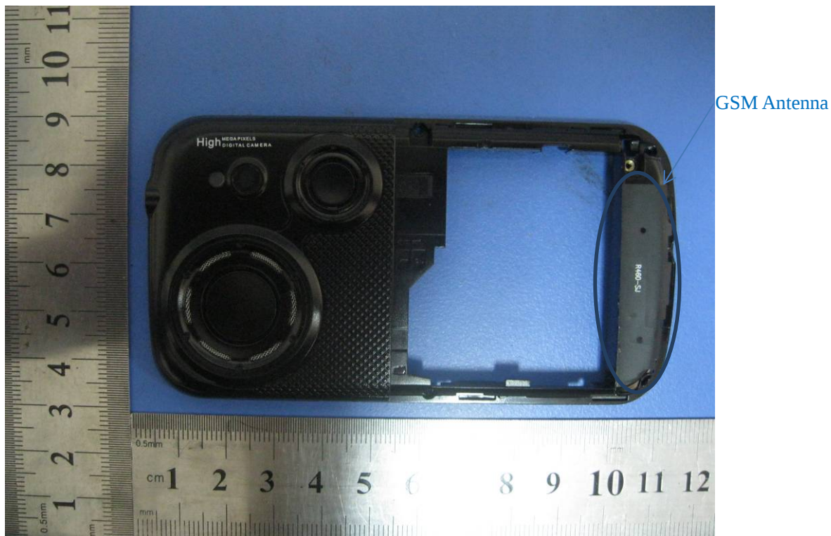
GSM Antenna - Top View
