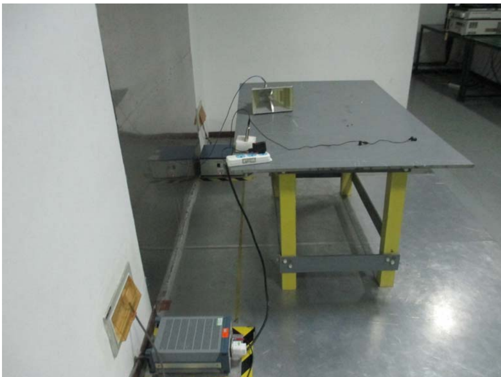
Conducted Emissions Test Setup Side View
