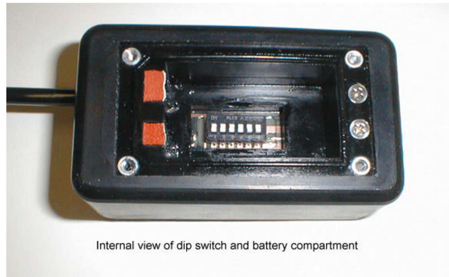
Internal view of dip switch and battery compartment
