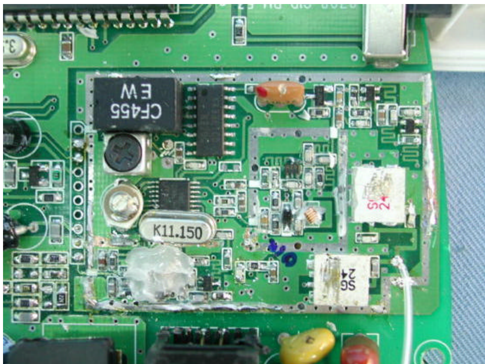
Base Oscillator PCB comp side
