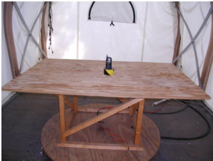
**Handset Radiated Emission - Rear View**
