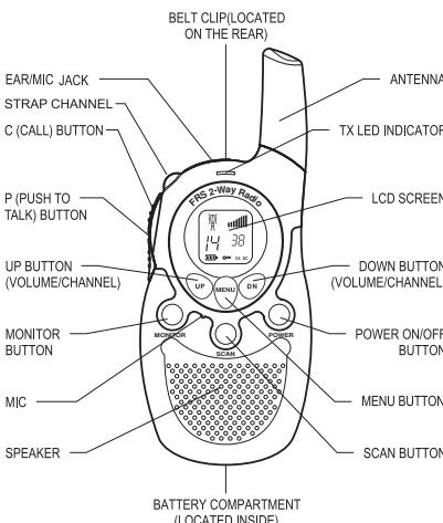
**LCD (Liquid Crystal Display)** - A multi-functional display, which shows channel, code and other radio status/icons (see specifics below).
