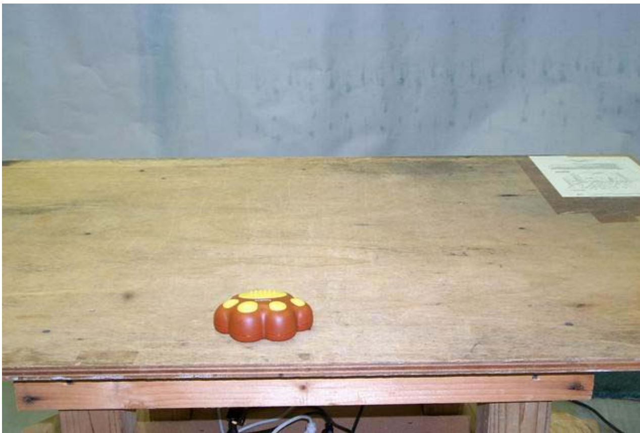
Figure 3.2 Radiated Test Setup, Rear
