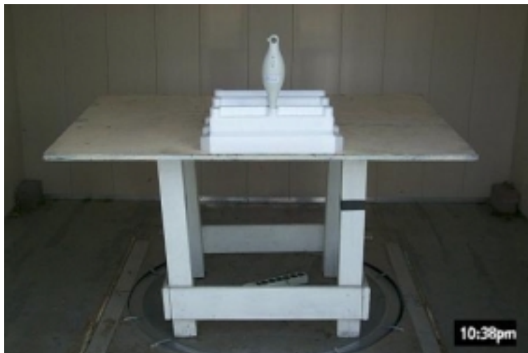
Figure 3.1 Radiated Test Setup, Front
