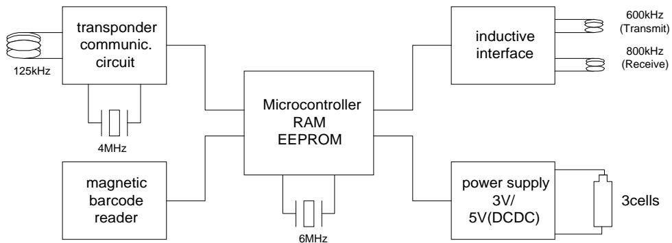
Most functions are performed by the micro-controller (80C154) operating at a clock frequency of **6MHz**. It is only active if necessary – otherwise it is in standby mode (oscillator is off).
