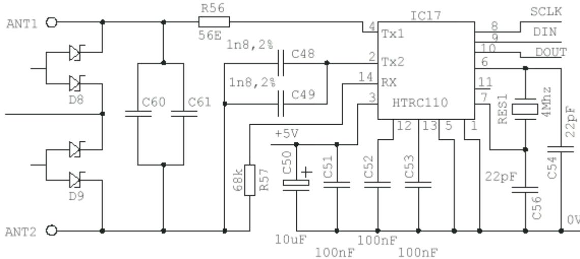
The antenna circuit is similar to the minimal required circuit of the application note of the HTRC110.
