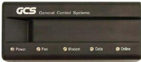
The GCS Pen **DTU** is the connection between the GCS **ProxiPen** and a PC or a modem.
