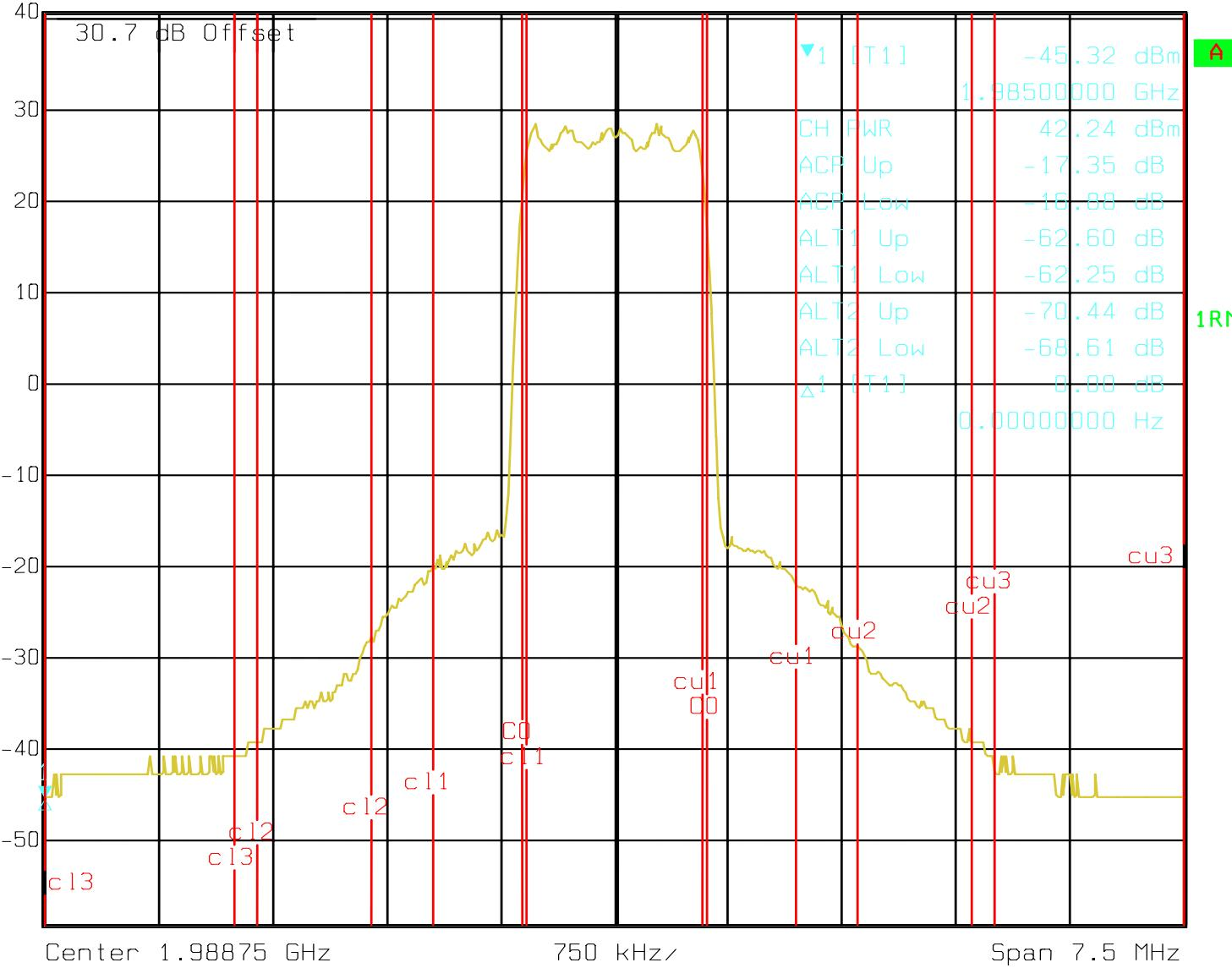
Name of Test: Spurious Emissions at Antenna Terminals
