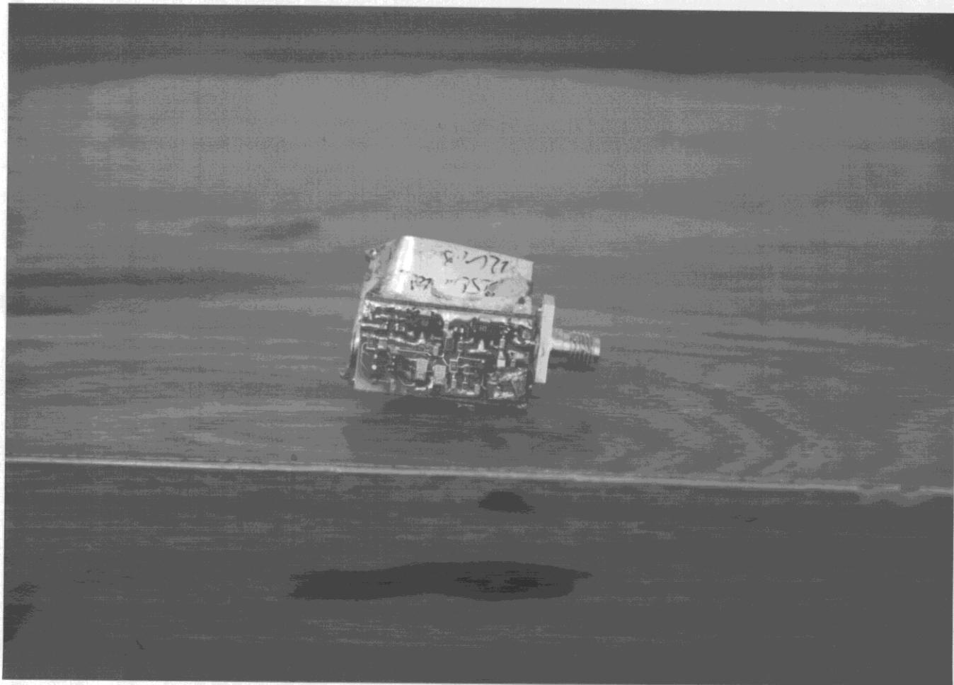
**Photograph of Component Side of Circuit Board with all Shielding Removed**
