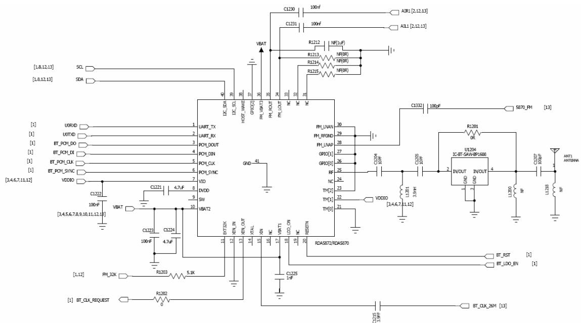
The Blue tooth over all schematic as up.RDA5872 is a highly integrated Bluetooth IC, which is compliant with Bluetooth2.0 specification and provides an optimal solution for data and voice application. It includes powerful processing capabilities with rich features and a high performance transceiver, all in a compact single package.
