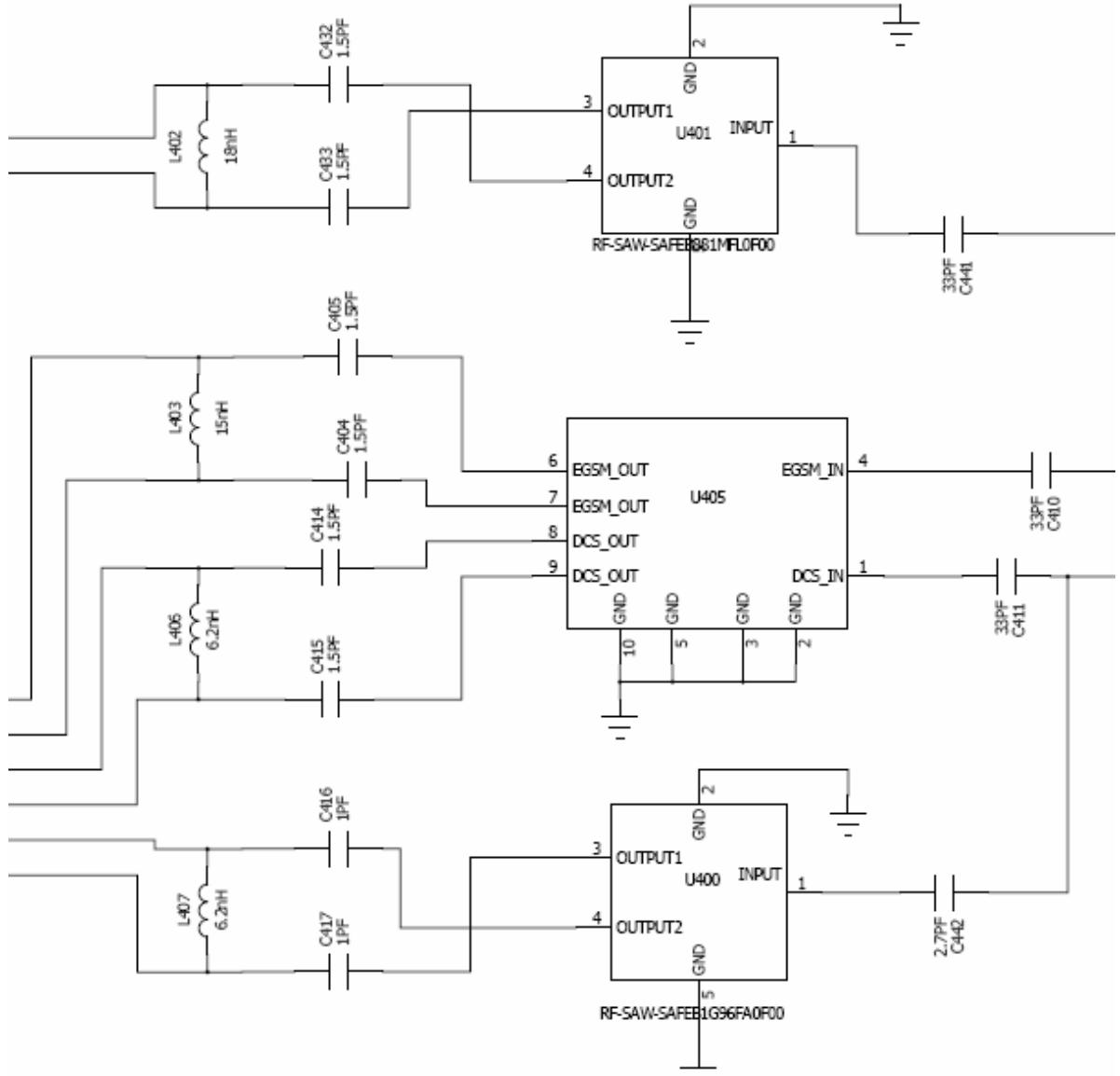
The RX signal output from RF SW, then input SAW filter, changed two difference signal in SAW filter,
