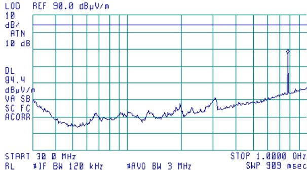
**Plot 7.5.6 Radiated emission measurements in 30 - 1000 MHz range**
