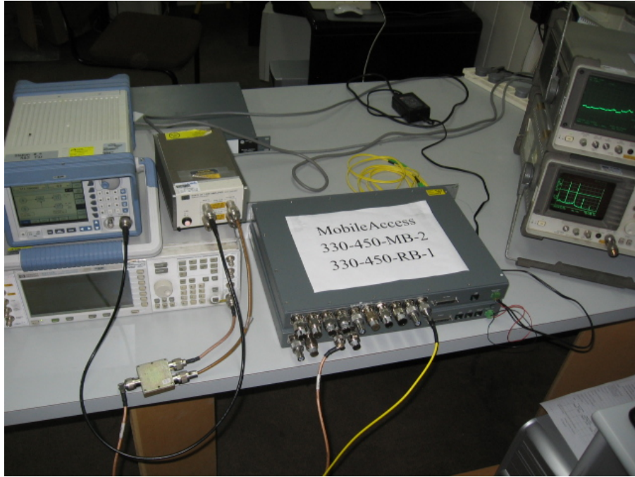
Figure 7. Conducted Emission From Antenna Ports Tests
