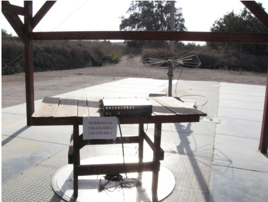
Figure 5. Radiated Emission Test
