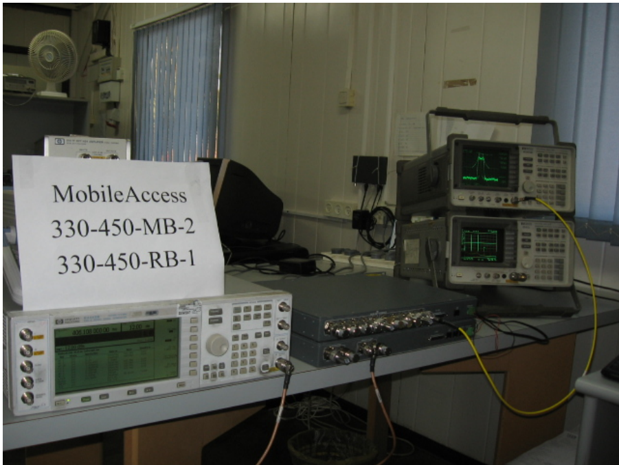
Figure 8. Conducted Emission From Antenna Ports Tests
