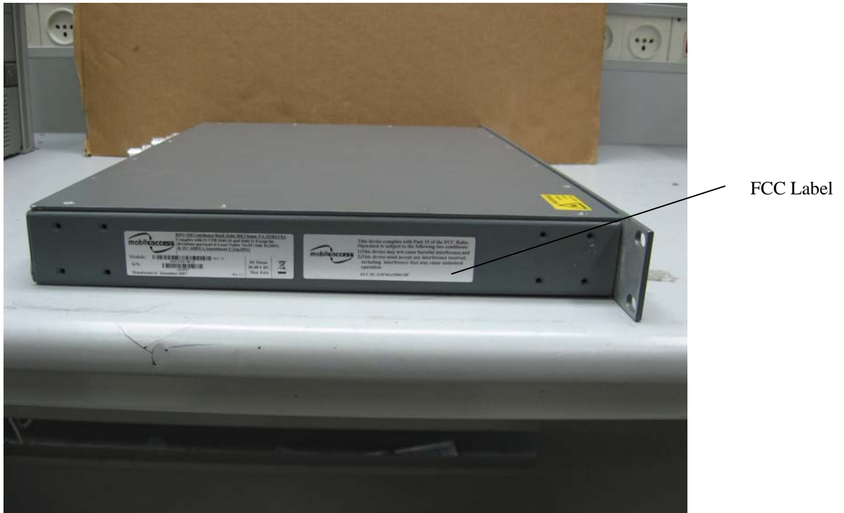
Figure 2. Label Location on the 1500-UHF-BU-2
