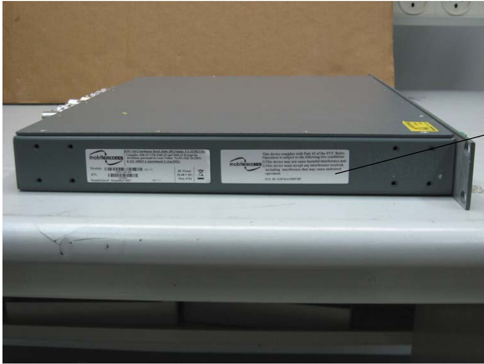
Figure 3. Label Location on the 1500-UHF-RU
