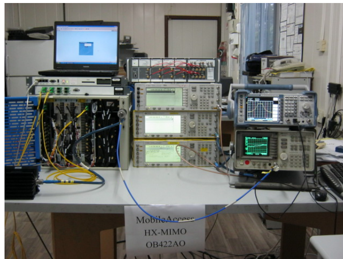
Figure 3. Conducted Emission From Antenna Ports Tests
