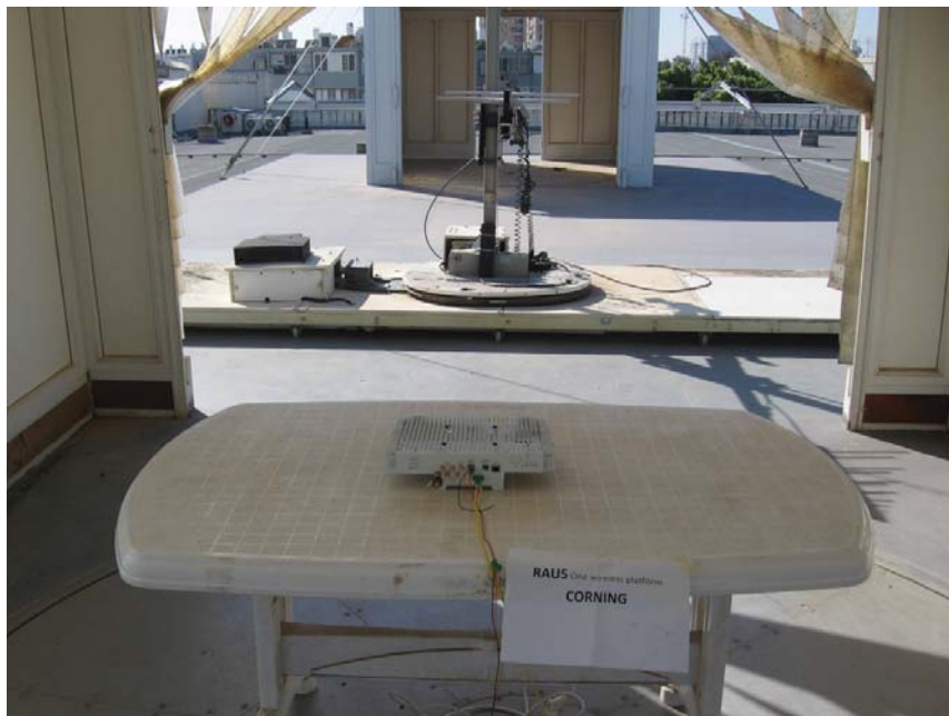
Figure 6. Radiated Emission Test
