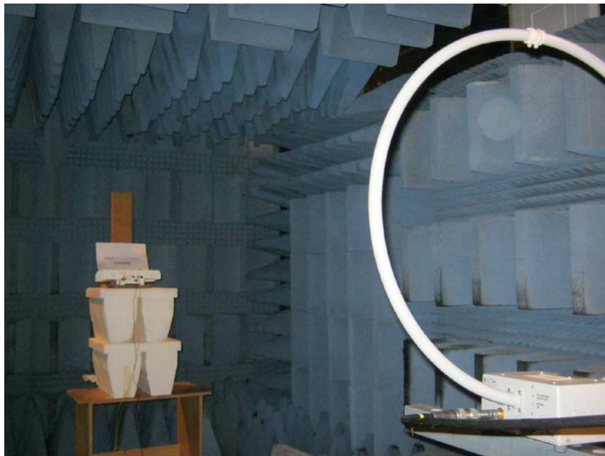
Figure 8. Radiated Emission Test
