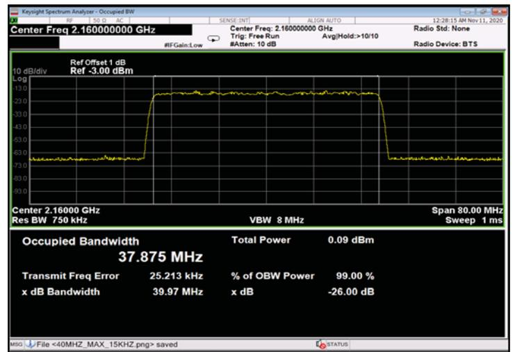
Figure 454: 256QAM 40MHz B.W.; 2160.0MHz, 30kHz - Input
