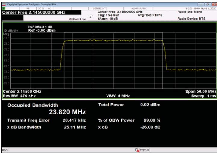
Figure 441: 256QAM 25MHz B.W.; 2145.0MHz, 15kHz - Input
