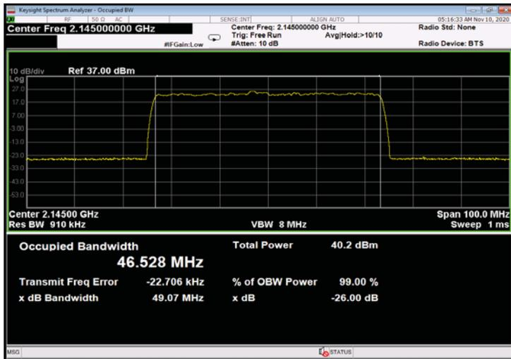
Figure 395: 64QAM 50MHz B.W.; 2145.0MHz, 60kHz - Input
