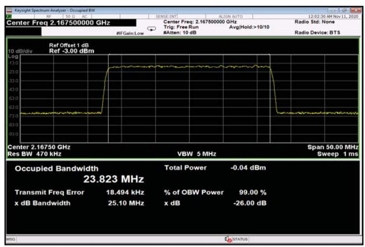
Figure 444: 256QAM 25MHz B.W.; 2167.5MHz, 15kHz - Input
