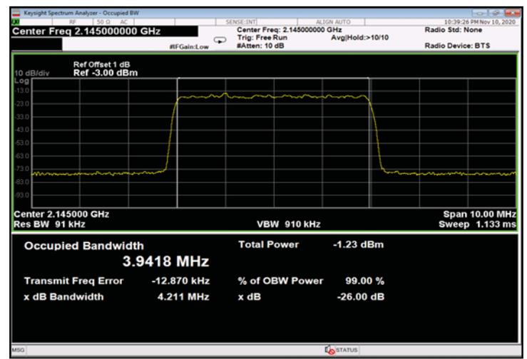
Figure 408: 256QAM 5MHz B.W.; 2145.0MHz, 30kHz - Input
