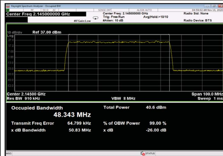
Figure 393: 64QAM 50MHz B.W.; 2145.0MHz, 15kHz - Input
