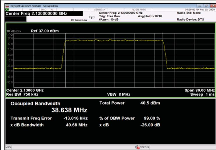
Figure 381: 64QAM 40MHz B.W.; 2130.0MHz, 15kHz – Input
