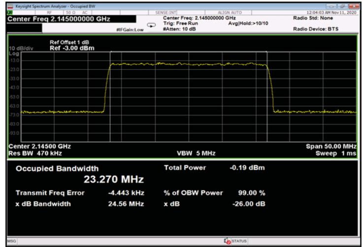
Figure 442: 256QAM 25MHz B.W.; 2145.0MHz, 30kHz - Input
