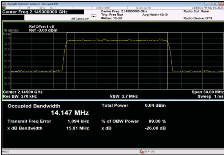
Figure 423: 256QAM 15MHz B.W.; 2145.0MHz, 15kHz - Input
