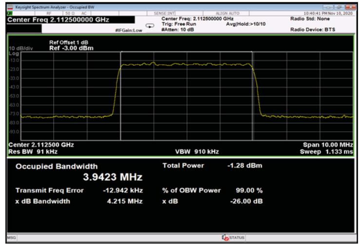
Figure 406: 256QAM 5MHz B.W.; 2112.5MHz, 30kHz - Input
