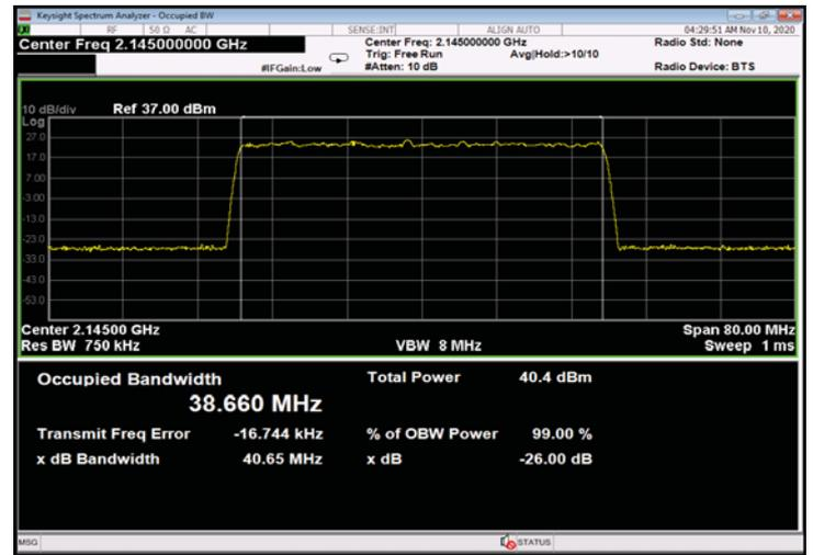
Figure 384: 64QAM 40MHz B.W.; 2145.0MHz, 15kHz - Input
