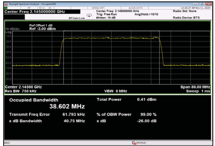
Figure 450: 256QAM 40MHz B.W.; 2145.0MHz, 15kHz - Input
