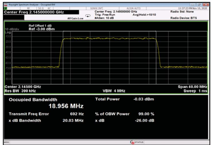
Figure 432: 256QAM 20MHz B.W.; 2145.0MHz, 15kHz - Input
