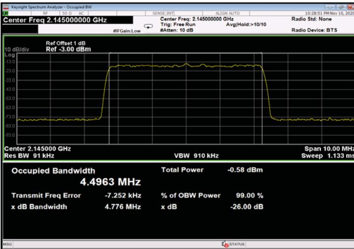
Figure 407: 256QAM 5MHz B.W.; 2145.0MHz, 15kHz - Input
