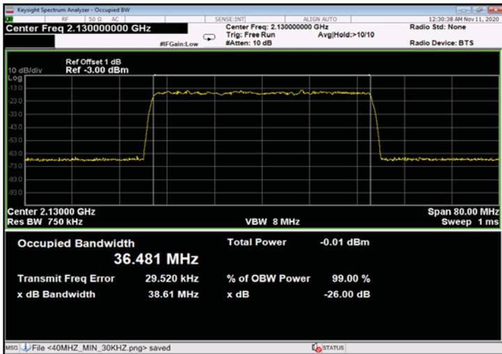
Figure 449: 256QAM 40MHz B.W.; 2130.0MHz, 60kHz - Input
