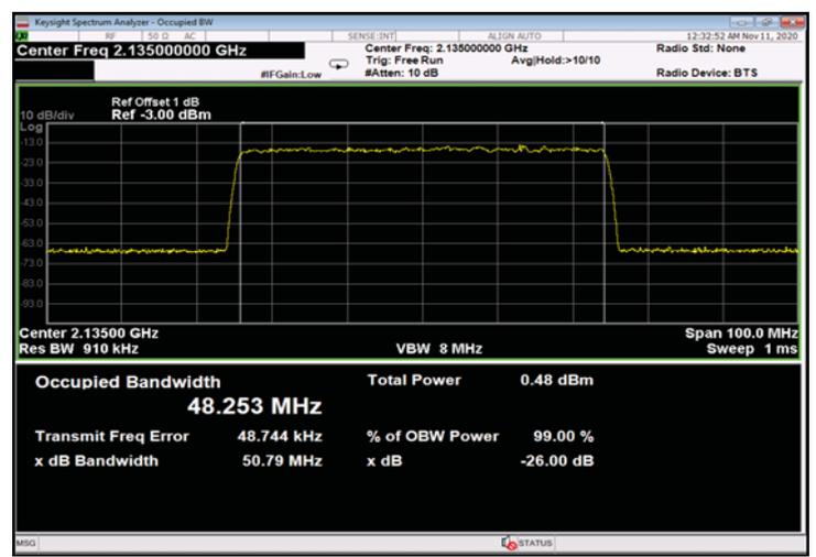
Figure 456: 256QAM 50MHz B.W.; 2135.0MHz, 15kHz - Input
