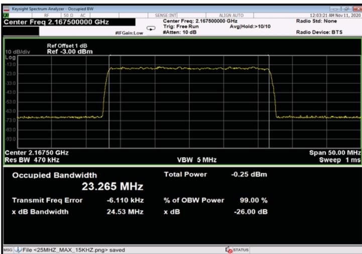
Figure 445: 256QAM 25MHz B.W.; 2167.5MHz, 30kHz - Input
