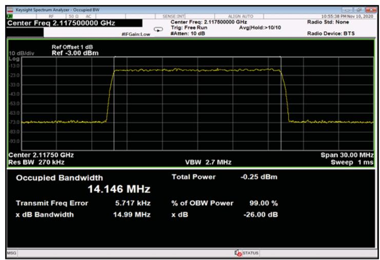
Figure 420: 256QAM 15MHz B.W.; 2117.5MHz, 15kHz - Input
