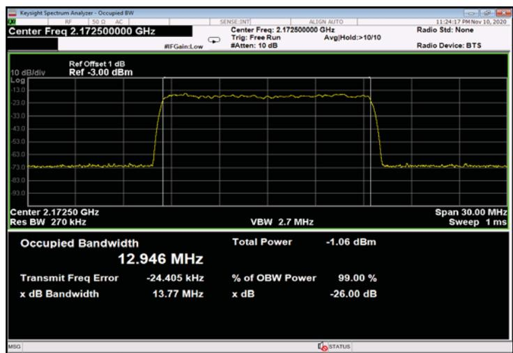
Figure 428: 256QAM 15MHz B.W.; 2172.5MHz, 60kHz - Input
