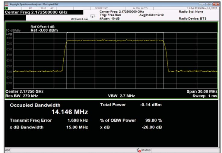
Figure 426: 256QAM 15MHz B.W.; 2172.5MHz, 15kHz - Input
