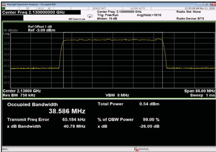
Figure 447: 256QAM 40MHz B.W.; 2130.0MHz, 15kHz - Input
