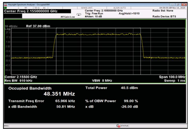
Figure 396: 64QAM 50MHz B.W.; 2155.0MHz, 15kHz - Input
