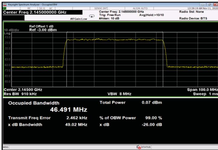
Figure 461: 256QAM 50MHz B.W.; 2145.0MHz, 60kHz - Input
