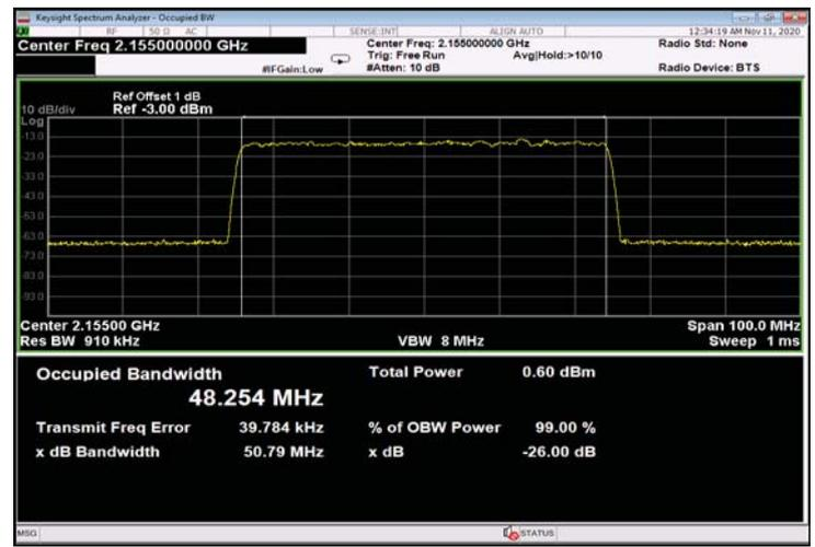
Figure 462: 256QAM 50MHz B.W.; 2155.0MHz, 15kHz - Input
