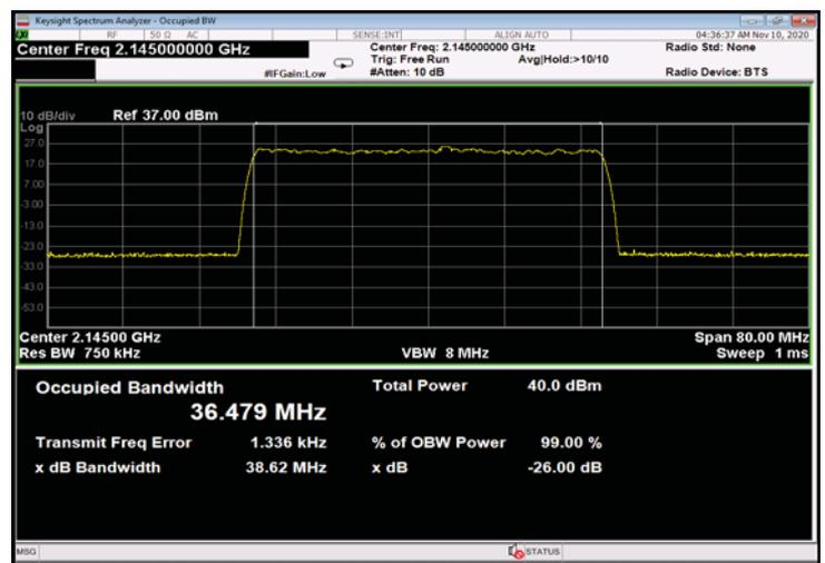
Figure 386: 64QAM 40MHz B.W.; 2145.0MHz, 60kHz - Input
