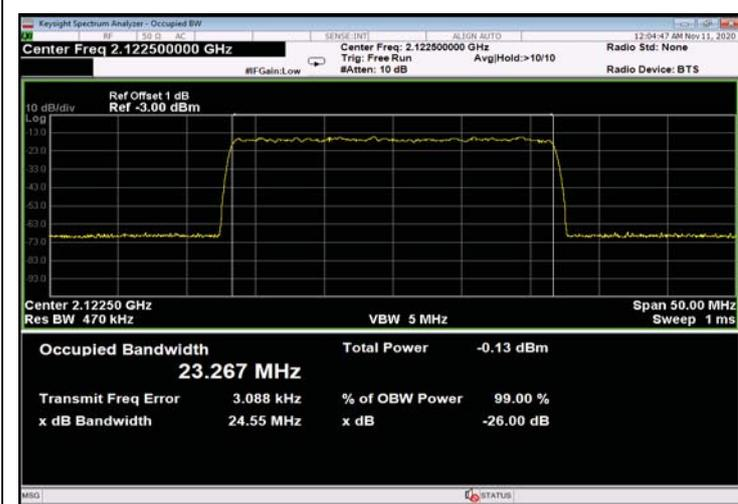
Figure 439: 256QAM 25MHz B.W.; 2122.5MHz, 30kHz - Input
