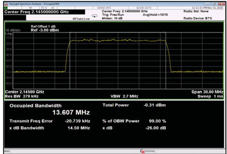
Figure 424: 256QAM 15MHz B.W.; 2145.0MHz, 30kHz - Input
