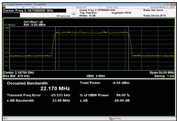
Figure 446: 256QAM 25MHz B.W.; 2167.5MHz, 60kHz - Input
