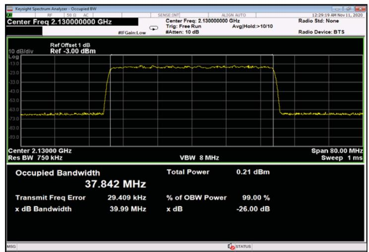
Figure 448: 256QAM 40MHz B.W.; 2130.0MHz, 30kHz - Input
