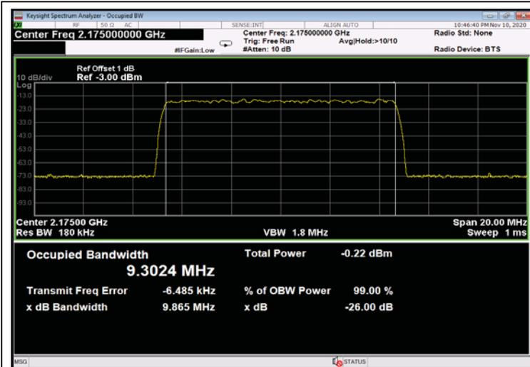
Figure 417: 256QAM 10MHz B.W.; 2175.0MHz, 15kHz - Input
