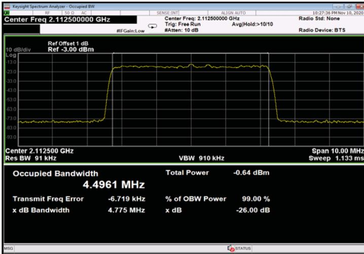
Figure 405: 256QAM 5MHz B.W.; 2112.5MHz, 15kHz - Input
