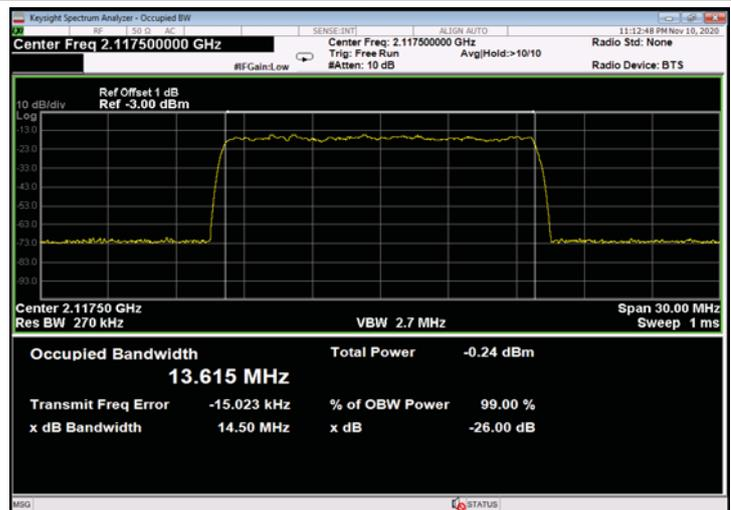
Figure 421: 256QAM 15MHz B.W.; 2117.5MHz, 30kHz - Input
