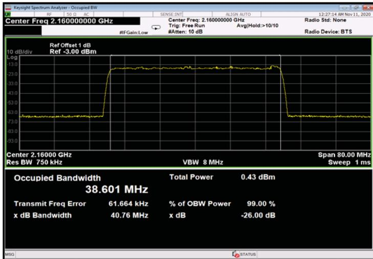
Figure 453: 256QAM 40MHz B.W.; 2160.0MHz, 15kHz - Input
