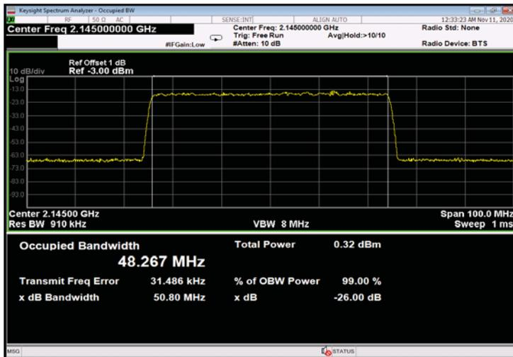
Figure 459: 256QAM 50MHz B.W.; 2145.0MHz, 15kHz - Input
