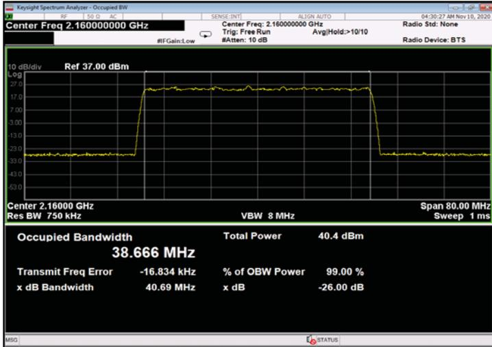
Figure 387: 64QAM 40MHz B.W.; 2160.0MHz, 15kHz - Input
