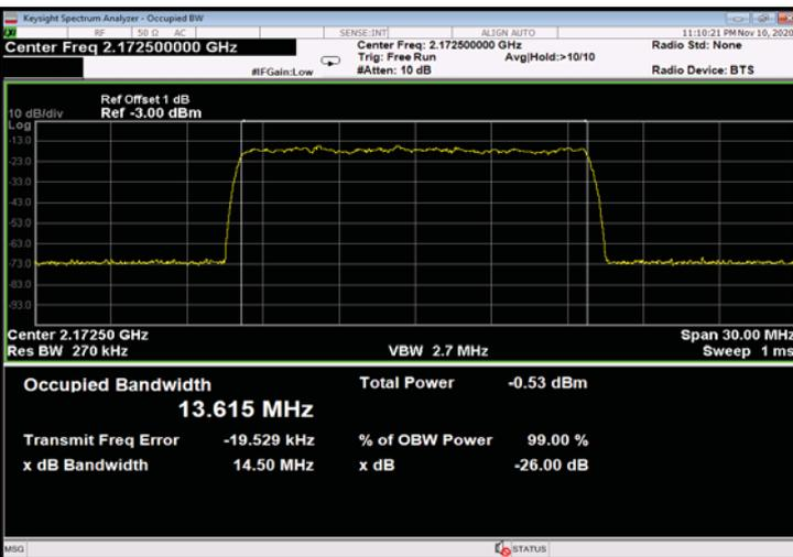
Figure 427: 256QAM 15MHz B.W.; 2172.5MHz, 30kHz - Input
