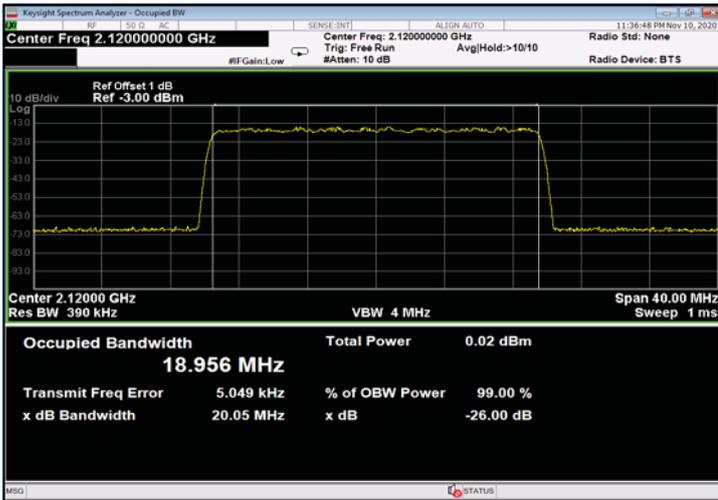
Figure 429: 256QAM 20MHz B.W.; 2120.0MHz, 15kHz - Input
