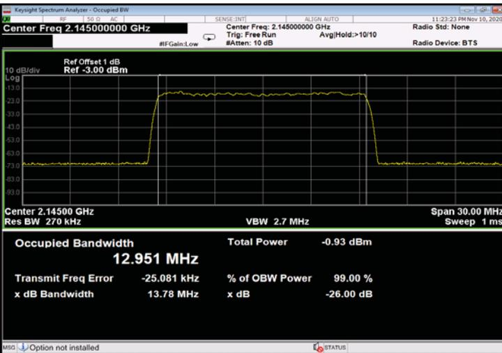
Figure 425: 256QAM 15MHz B.W.; 2145.0MHz, 60kHz - Input
