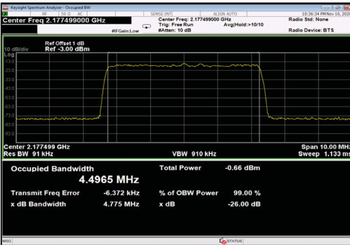
Figure 409: 256QAM 5MHz B.W.; 2177.5MHz, 15kHz - Input
