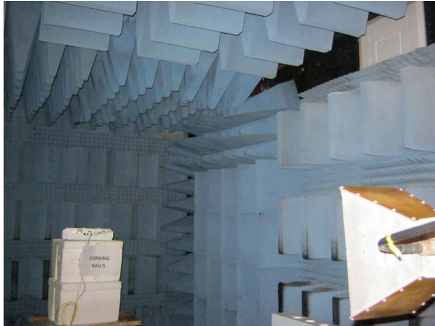
Figure 7. Radiated Emission Test
