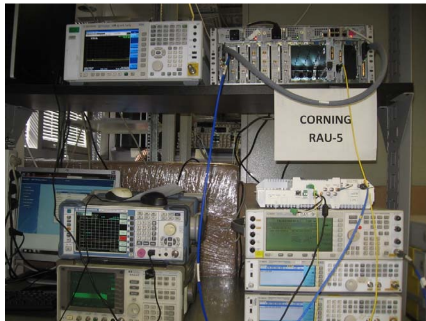
Figure 3. Conducted Emission From Antenna Port Tests
