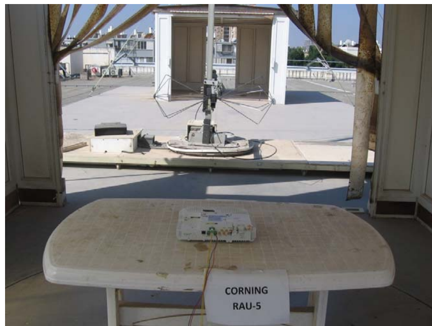
Figure 4. Radiated Emission Test
