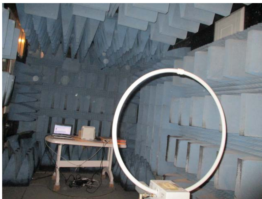
Figure 4. Radiated Emission Test, 0.009-30MHz
