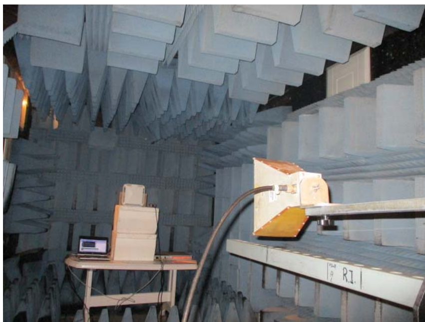
Figure 7. Radiated Emission Test, 1-18GHz
