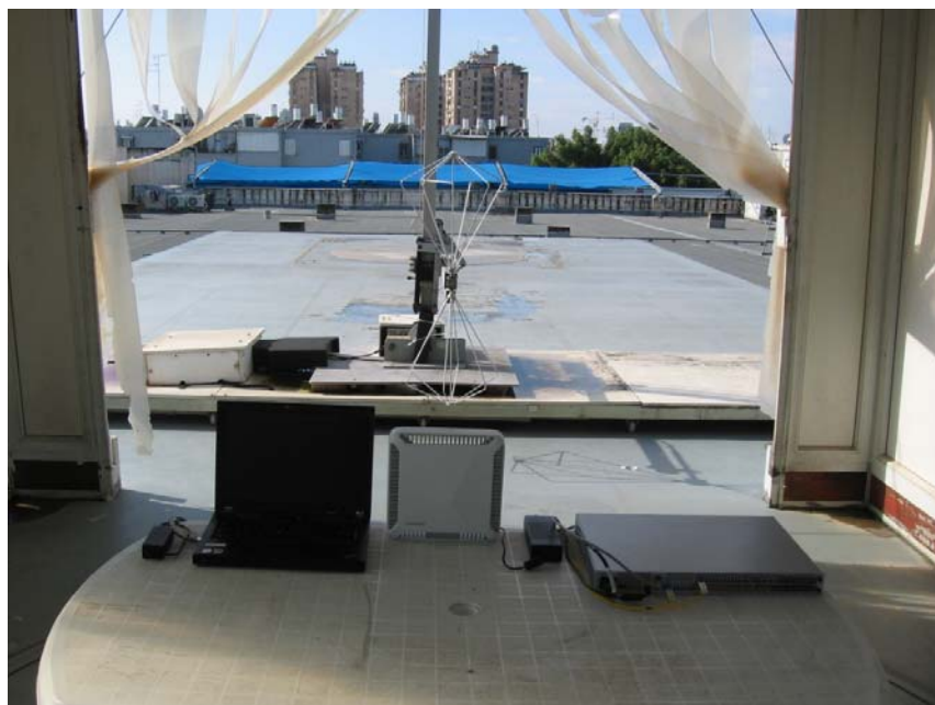
Figure 5. Radiated Emission Test, 30-200MHz
