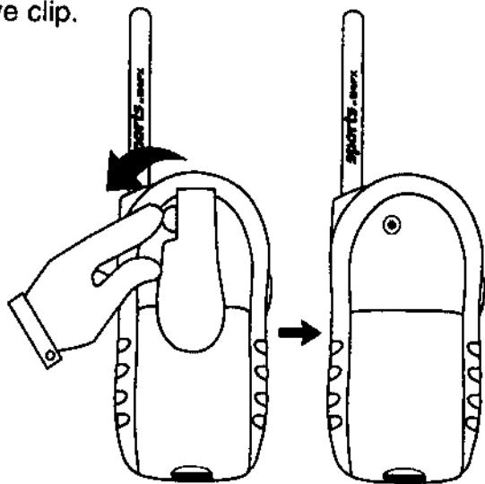
2. Align the screw and the clip with the screw hole and turn clockwise to attach clip. Do not overtighten the screw.
