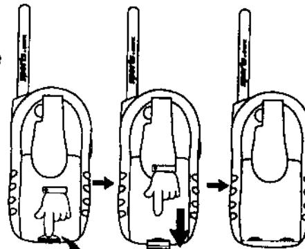
2. Insert (or remove) the 3 "AA" batteries.
