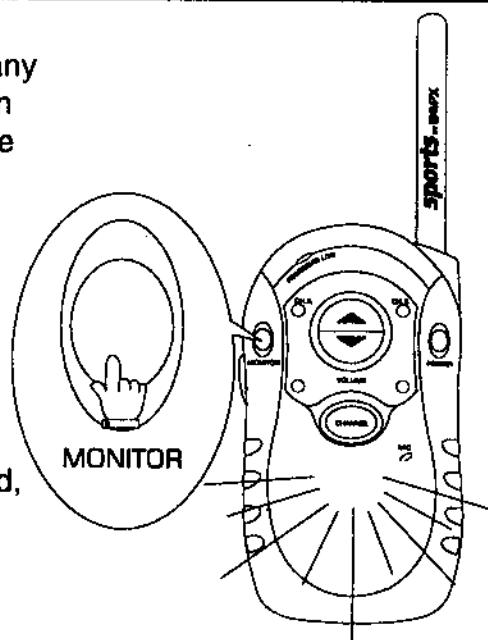
2. Press and hold the Monitor key. To deactivate the Monitor function.
