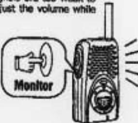
1. Press and hold the Monitor key for approximately 1 second to activate the Monitor function.
