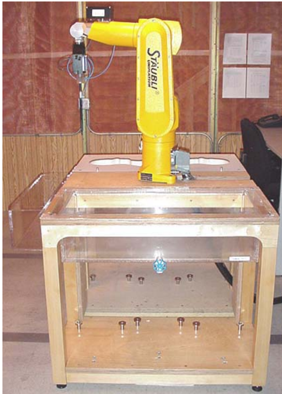
DASY4 SAR Measurement System with validation phantom
