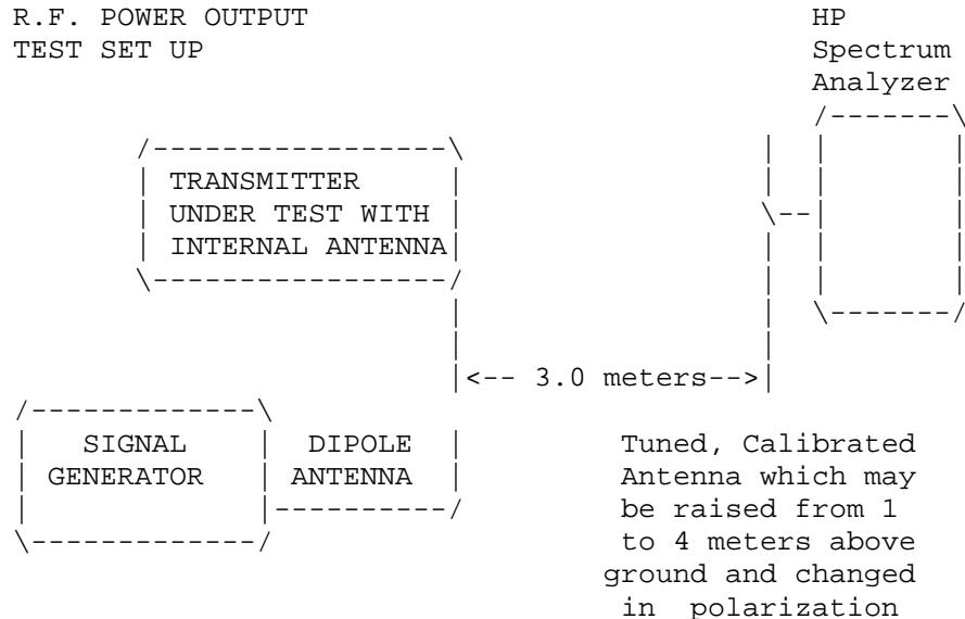
Equipment placed 1 meter above ground
