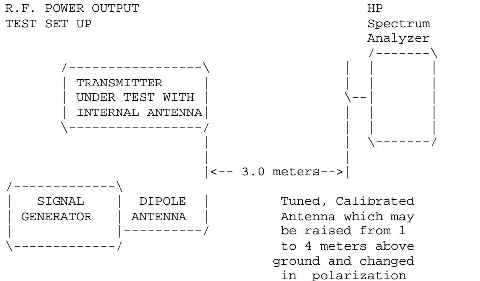
Equipment placed 1 meter above ground
