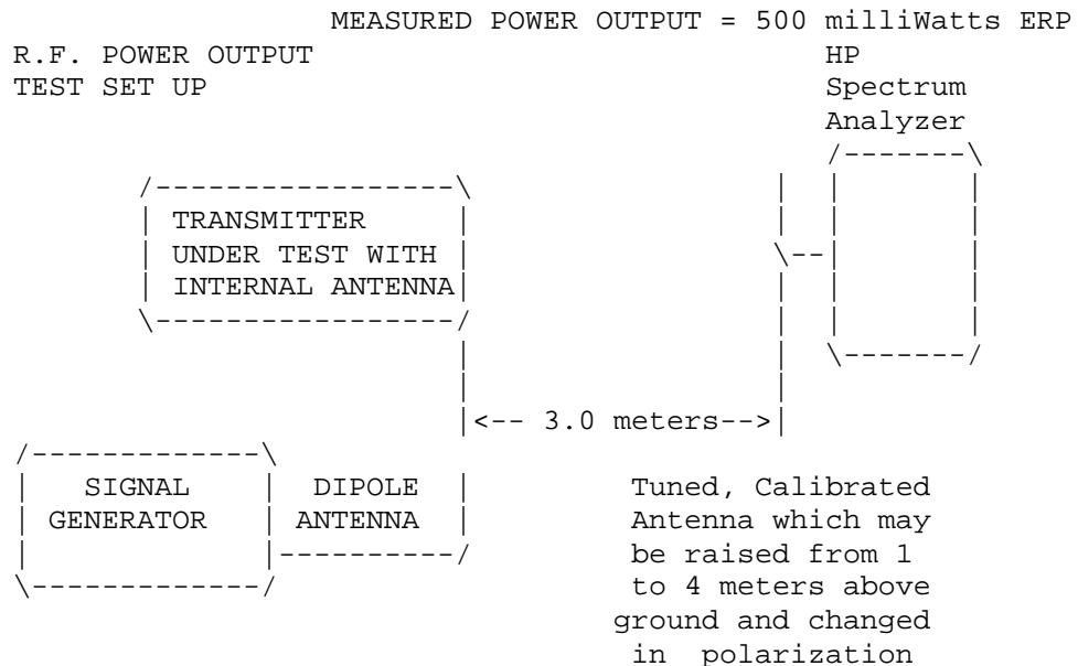
Equipment placed 1 meter above ground on a rotatable platform.
