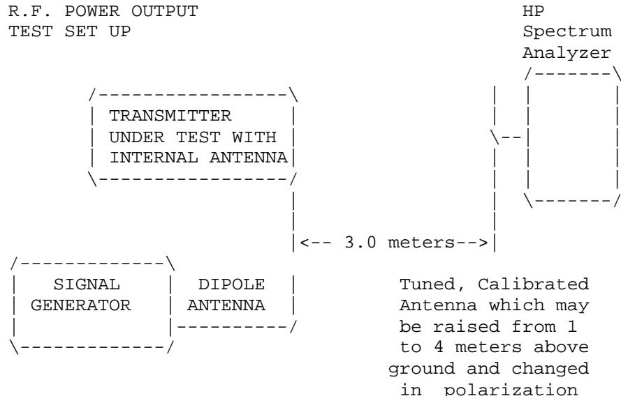
Equipment placed 1 meter above ground
