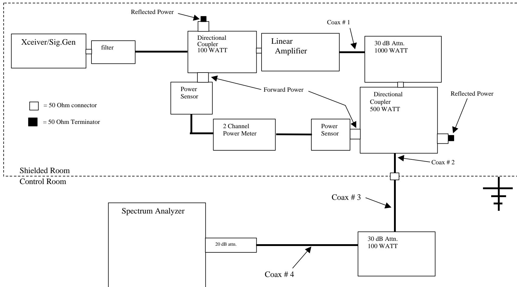
Correction Factor Power Meter Channel 1 = Attn. Directional Coupler Forward Power
