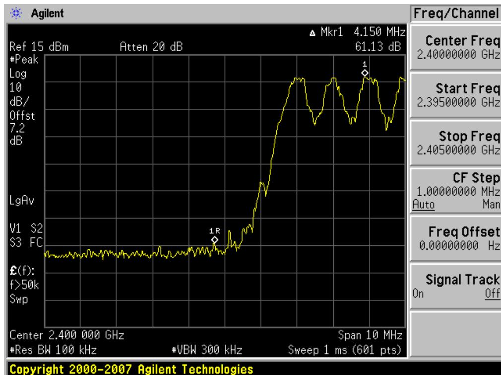
Test Plots with hopping (GFSK)
