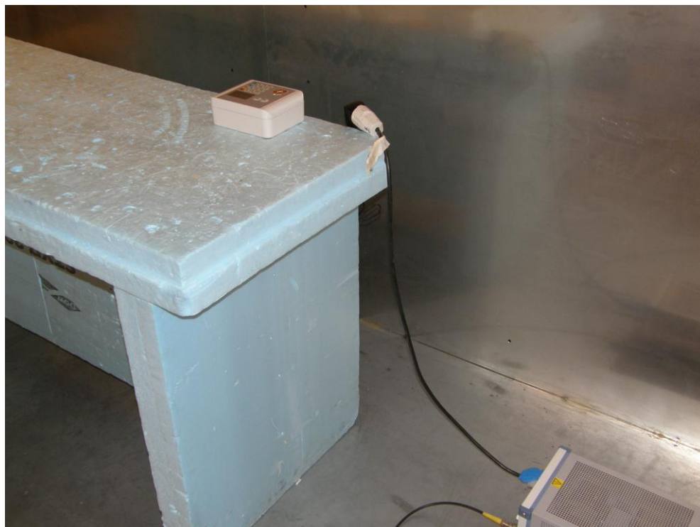
Photograph 2. Conducted disturbance at mains ports emission test.
