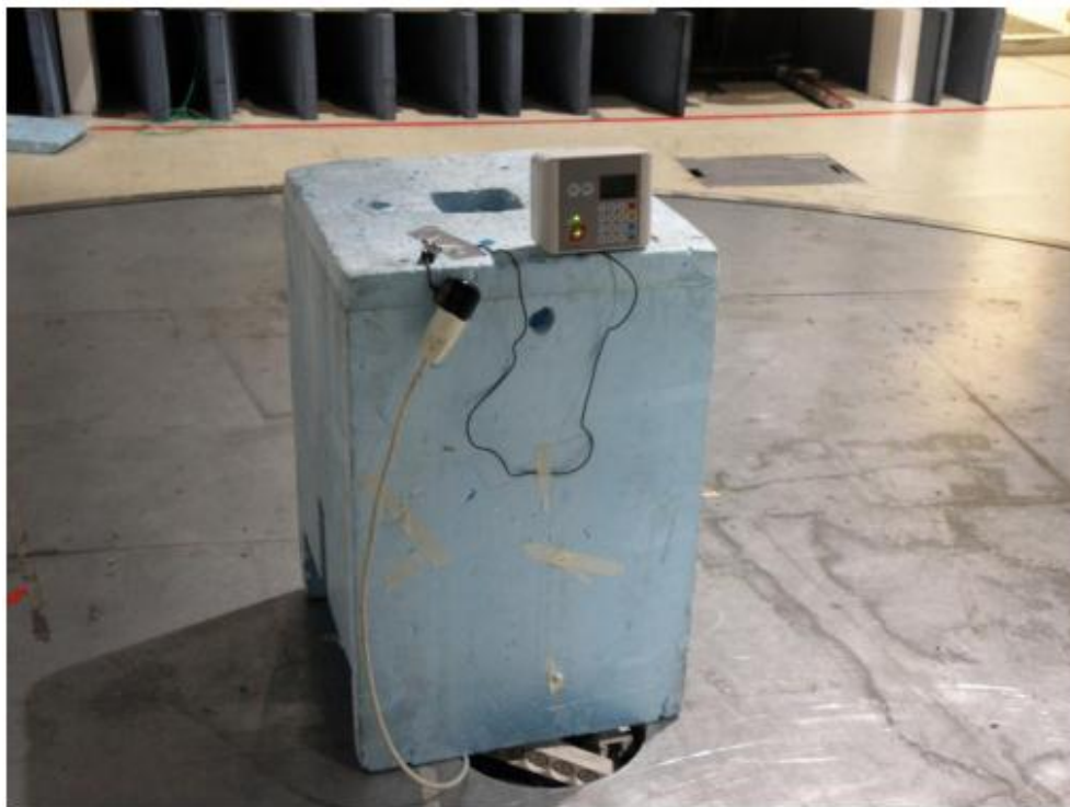
Photograph 1. Radiated spurious emission test 9 kHz – 1000 MHz.
