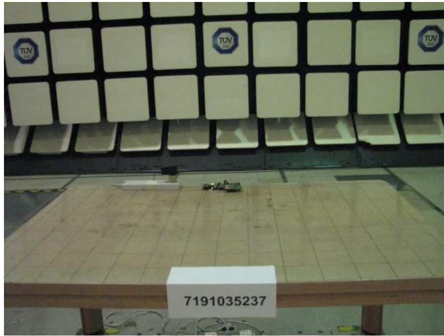
Radiated Emissions Test Setup (Front View)
