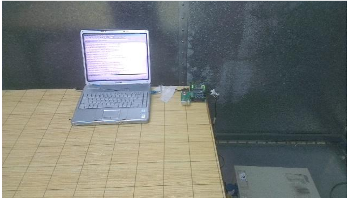
Conducted Emissions Test Setup (Front View)
