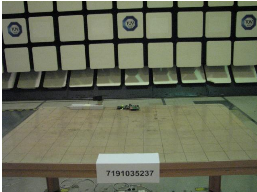
Radiated Emissions Test Setup (Front View)
