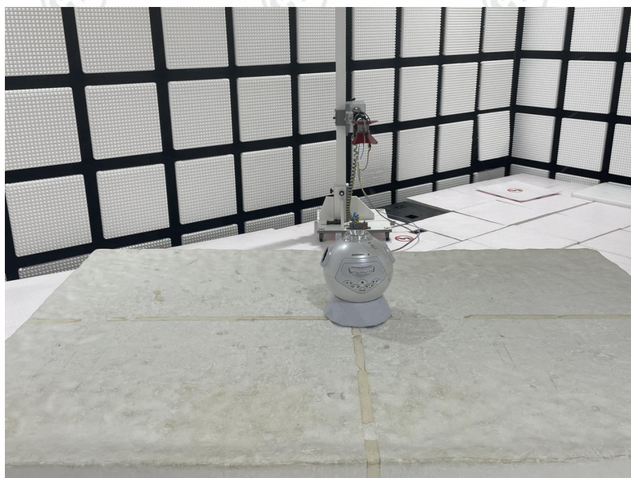
Radiated spurious emission Test Setup-2(Above 1GHz)
