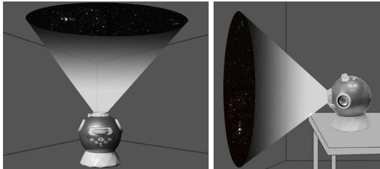
8. Adjust the focus dial (14) until the projected star field is sharp. The optimum project distance is 1.8m to 2m, image will become blur if the distance is too near or too far.
