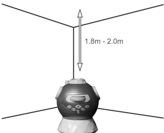
2. Place the unit over the stand(15) on a flat and stable platform (e.g. a table), the optimum project distance is about 1.8m to 2m.
