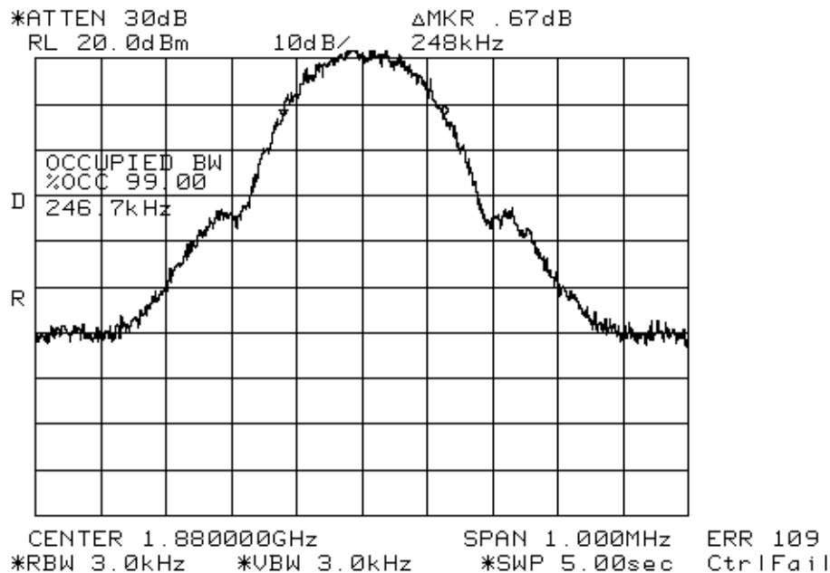
Figure E12.1. Sample RM measurement of occupied bandwidth.
