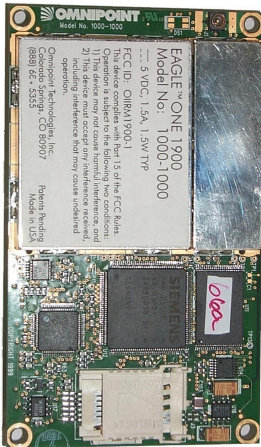
Photo 3. Top of RM PCB with RF shields covering radio circuitry.
