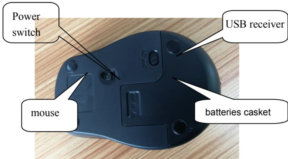
b. Put the batteries into the batteries casket, lock the cover.
