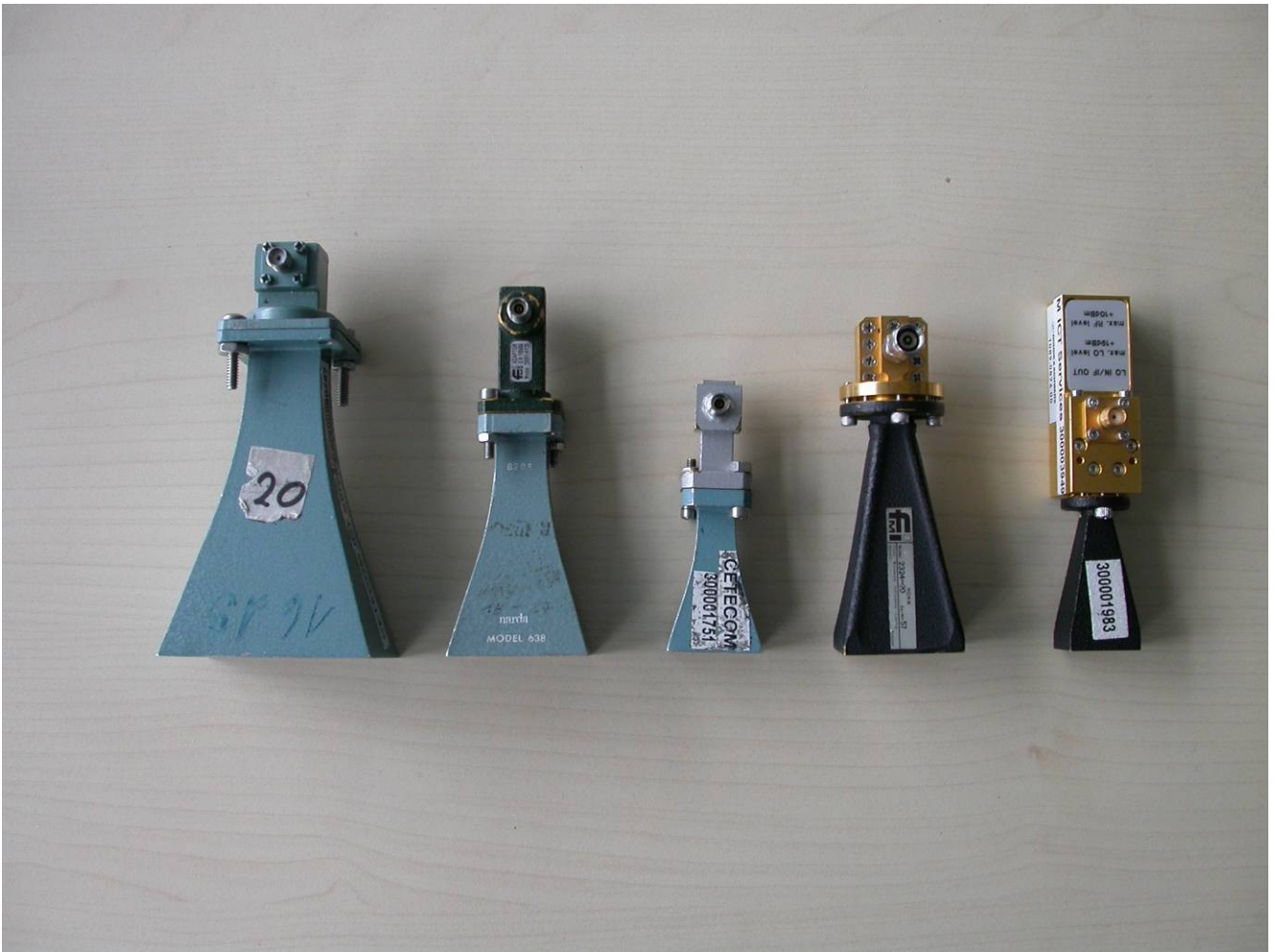
Spurious Emission test equipment 12 – 54 GHz
