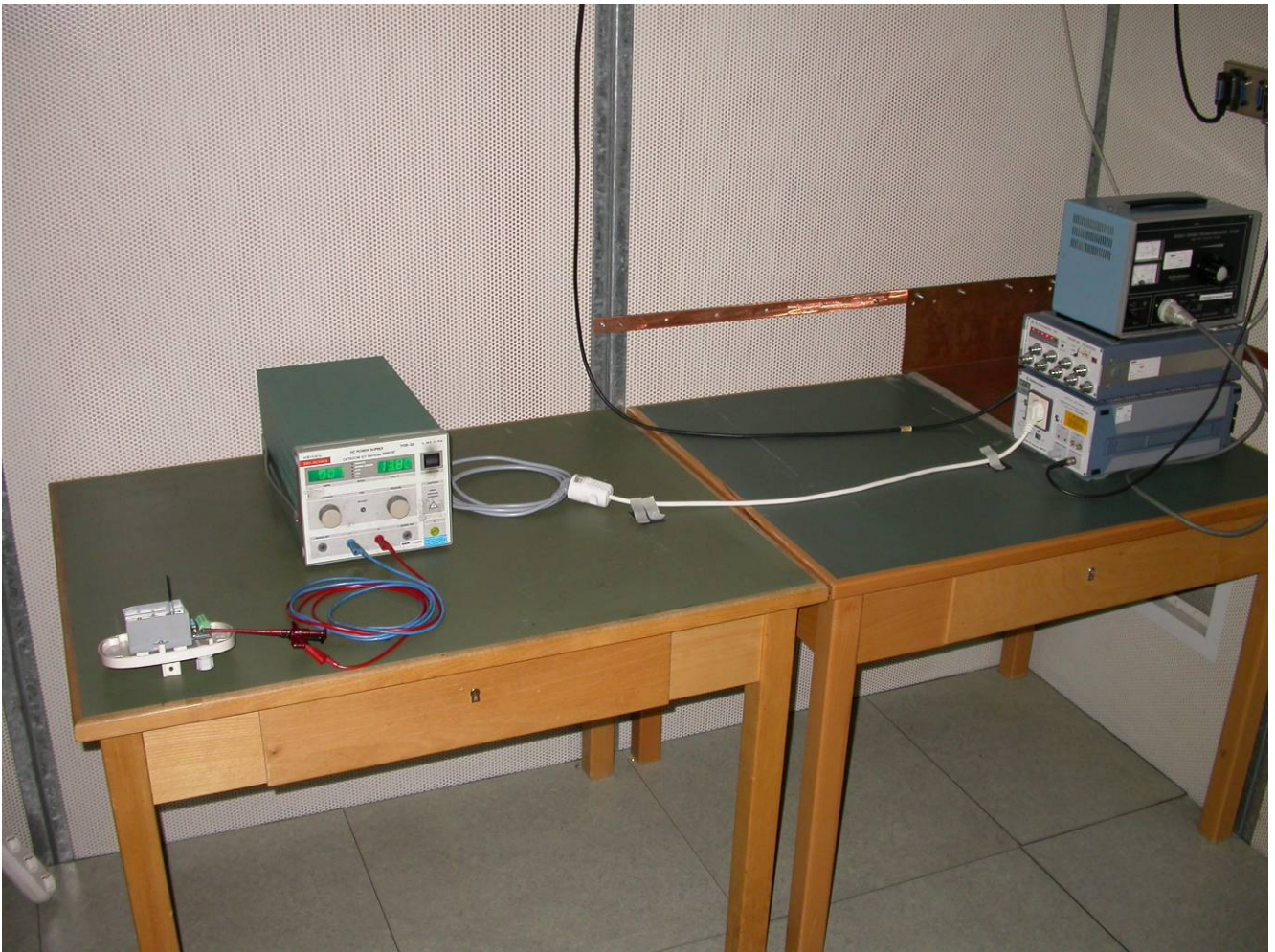
AC-conducted line measurement
