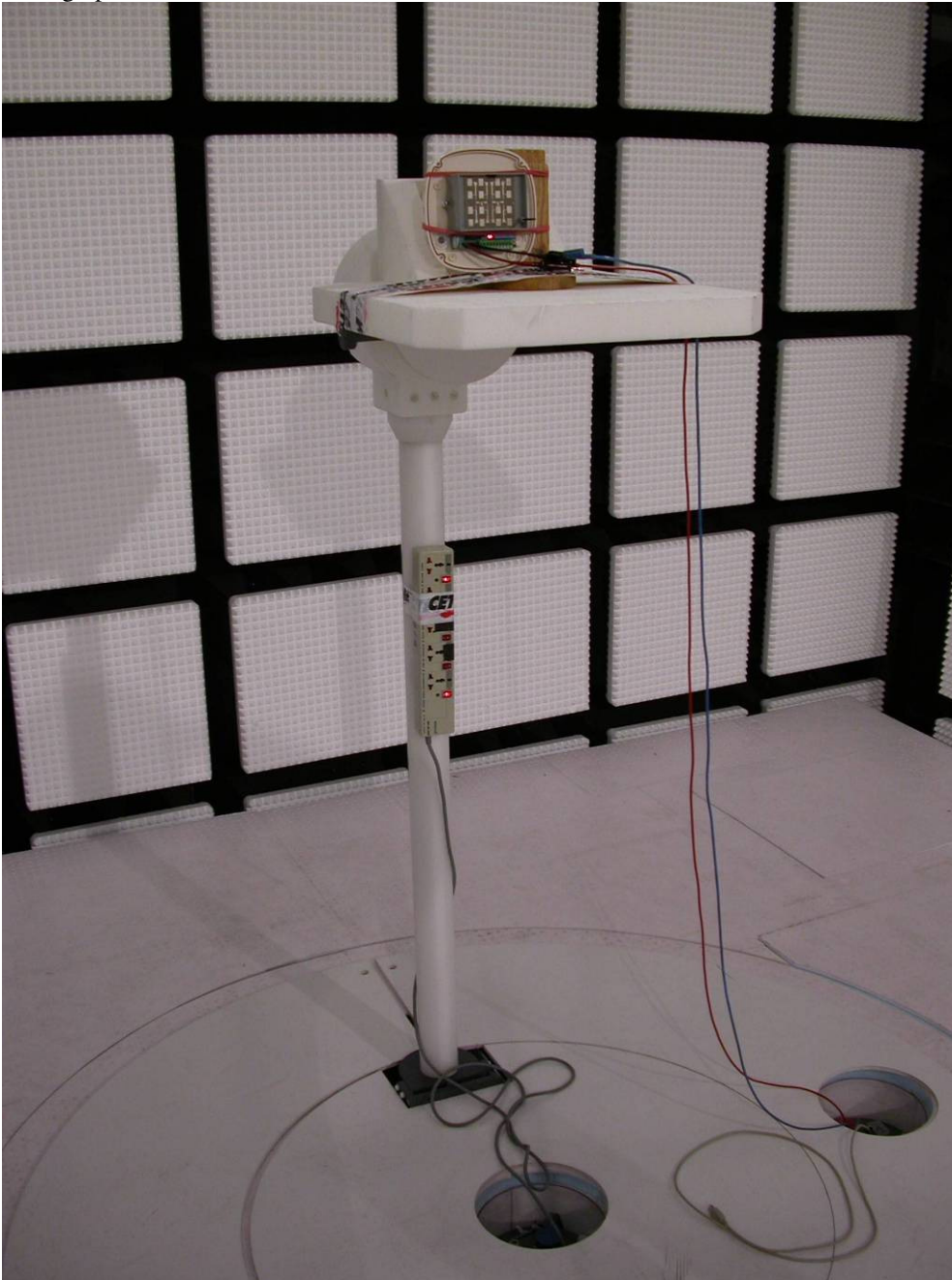
Spurious Emission measurement 1 GHz – 12 GHz
