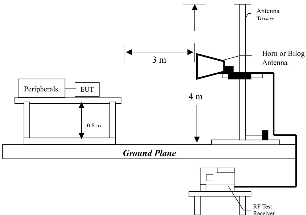
The signal is maximized through rotation and placement in the three orthogonal axes. The EUT and its peripherals are placed on a turn table which is 0.8 meter above ground. The turn table can rotate 360 degrees to determine the position of the maximum emission level. The EUT was positioned such that the distance from antenna to the EUT was 3 meters. The antenna can move up and down between 1 meter and 4 meters to find out the maximum emission level.
