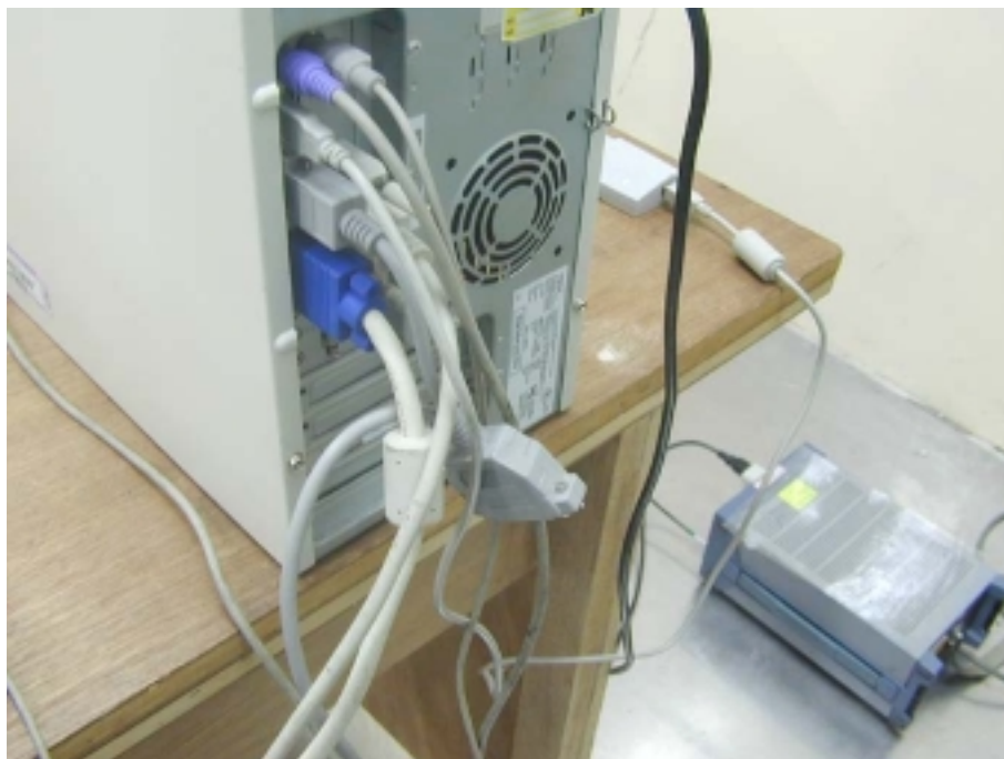
Photo 4: Conducted Test Set-up (enlarge)
