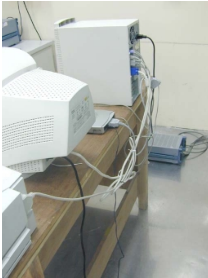
Photo 3: Conducted Test Set-up (rear view)
