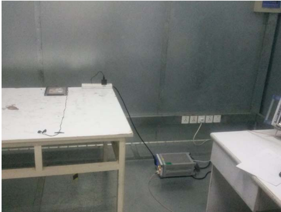
Set-up for Conducted Emission Test
