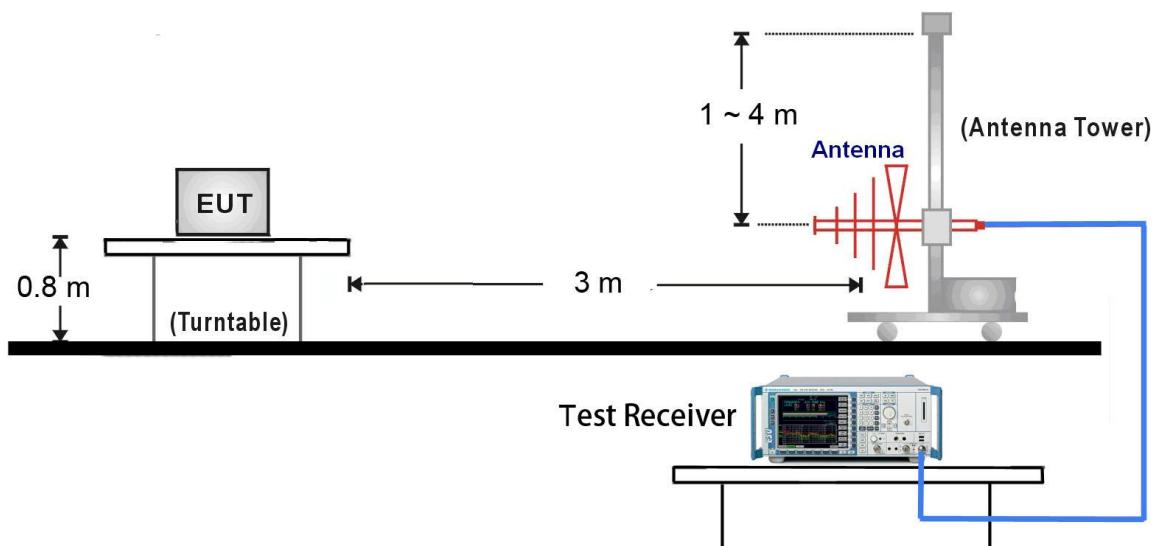
1GHz ~25GHz Test Setup:
