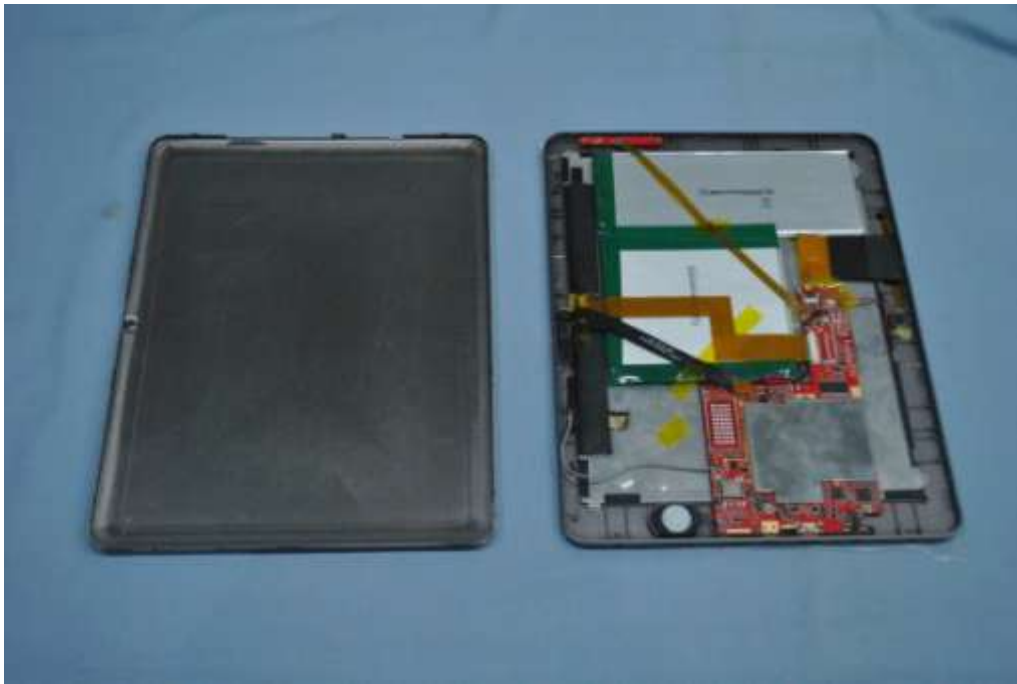
Main &amp; RF board component side
