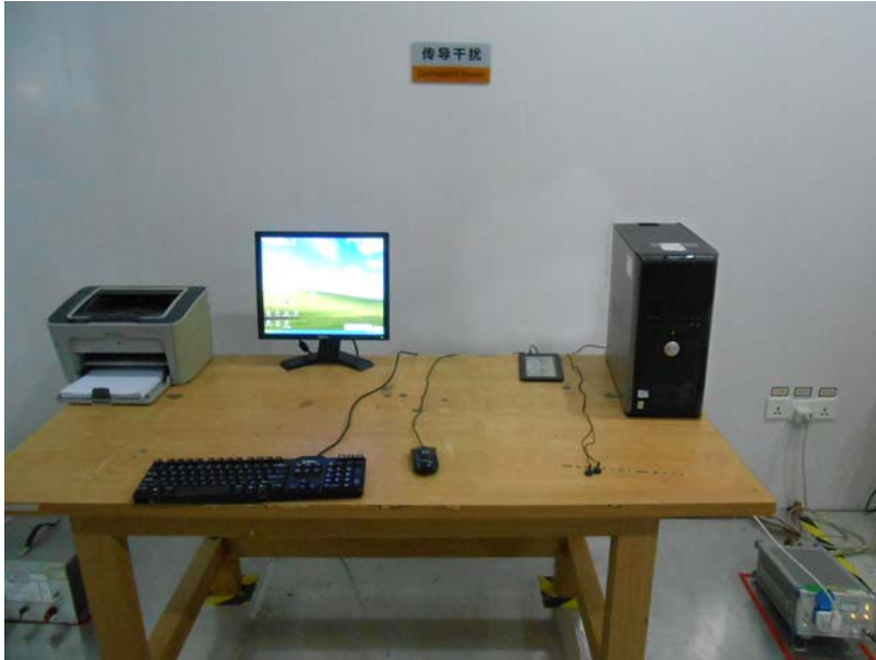
Photo of Setup for Conducted Emission
