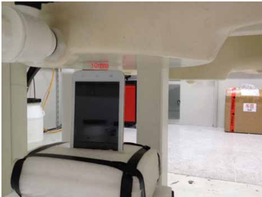
Body SAR Bottom 10mm for GSM/UMTS
