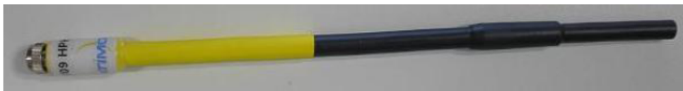
Figure 1 – Satimo COMOHAC H field Probe
